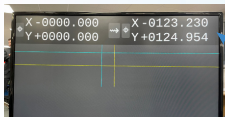
0.005mm micro positional adjustments easily made by the operator. Final position recorded in software
